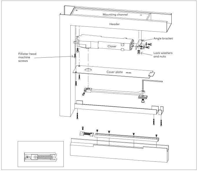
NOTE: 8532 mounting channel is to be installed prior to frame installion.
